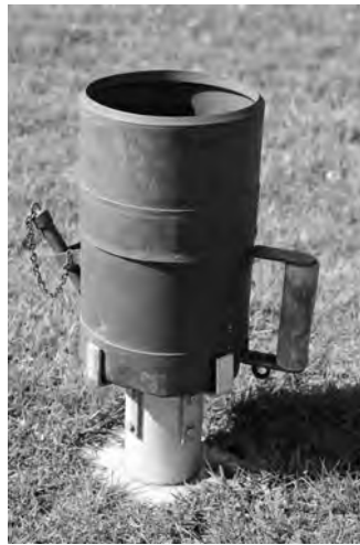
Figure 1.6: Example of a manual rain gauge as used by the volunteer network of KNMI (courtesy of Aart Overeem).
