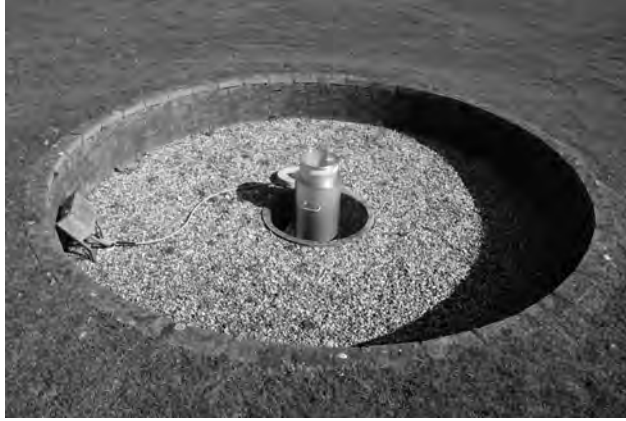
Figure 1.5: Example of an automatic rain gauge as operated by KNMI (courtesy of Aart Overeem).
