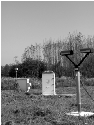
Figure 1.9: A 2-D video disdrometer (middle, with processing unit and sonic anemometer, left) and an optical disdrometer (right) at Cabauw, The Netherlands (courtesy of Hidde Leijnse).
